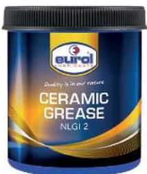
Ceramic Paste is especially formulated from high molecular oil, ceramic materials and inorganic thickener with additives. This Anti-Seize assembly paste has excellent lubricating properties and the strong adherence prevents water wash off. It can be used for all parts and threaded components which are usually treated with metal containing pastes like bearings, chains, fittings, splines, brake parts and pneumatic appliances, found in garages, ship building, agricultural and industrial plants.
